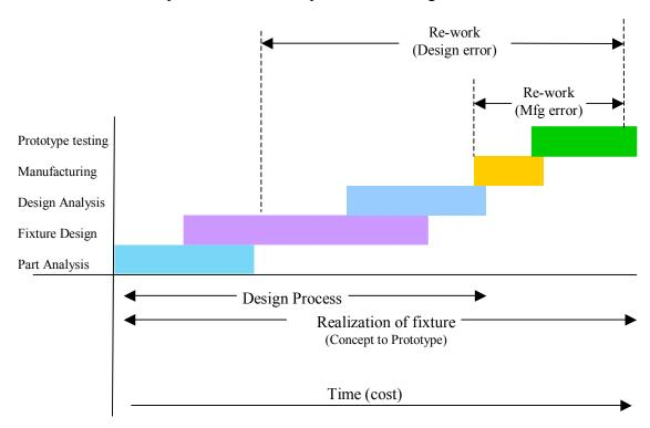
At every non-conformance point, (marked with red circles in the flow chart) the design cost shoots up non-linearly. The non-conformance cost in most cases is 100 % of what has been already encumbered or spent. The Gantt chart also shows the rework time spent due to design and manufacturing errors.
